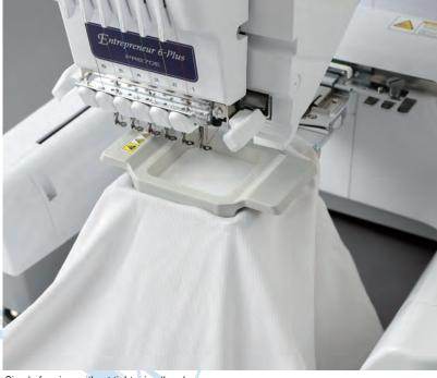
Simple framing, without tightening thumb screw.
